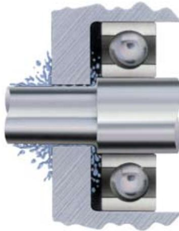
Without a viable bearing protection device installed, contaminants such as water, corrosive liquids, and dust/dirt can enter the bearings on pumps and electric motors. Costly bearing failures, motor rewindings, and production downtime are the result.
