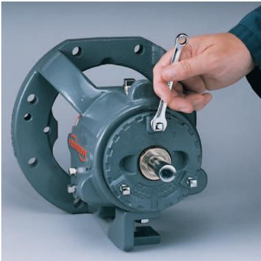
**Step 1:** Loosen the setscrews. Using a wrench rotate the bearing carrier counterclockwise until the impeller lightly touches the rear cover plate.
