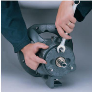
**Step 3:** Move the carrier clockwise the selected number of notches. Tighten the setscrews and check the impeller clearance with the feeler gauge.
