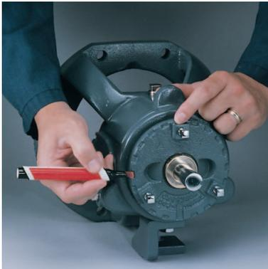
**Step 2:** Select the impeller setting. Each notch on the carrier ring represents exactly 0.10 mm (0.004 in) of clearance. For an impeller setting of 0.5 mm (0.020 in) count five notches counterclockwise.
