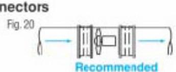
Flexible connectors should be just long enough for mechanical isolation and should be taut.
